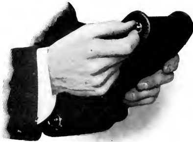
FIG. II. Springing Out a Spool Pin.
